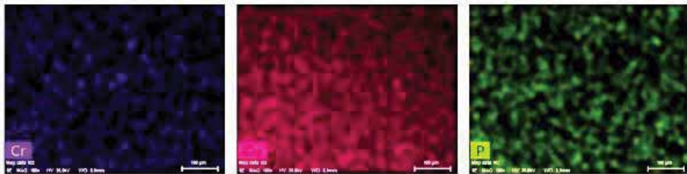
Figure 2. Distribution of Cu, Cr, and P in the CuCr0.6 alloy after casting.
