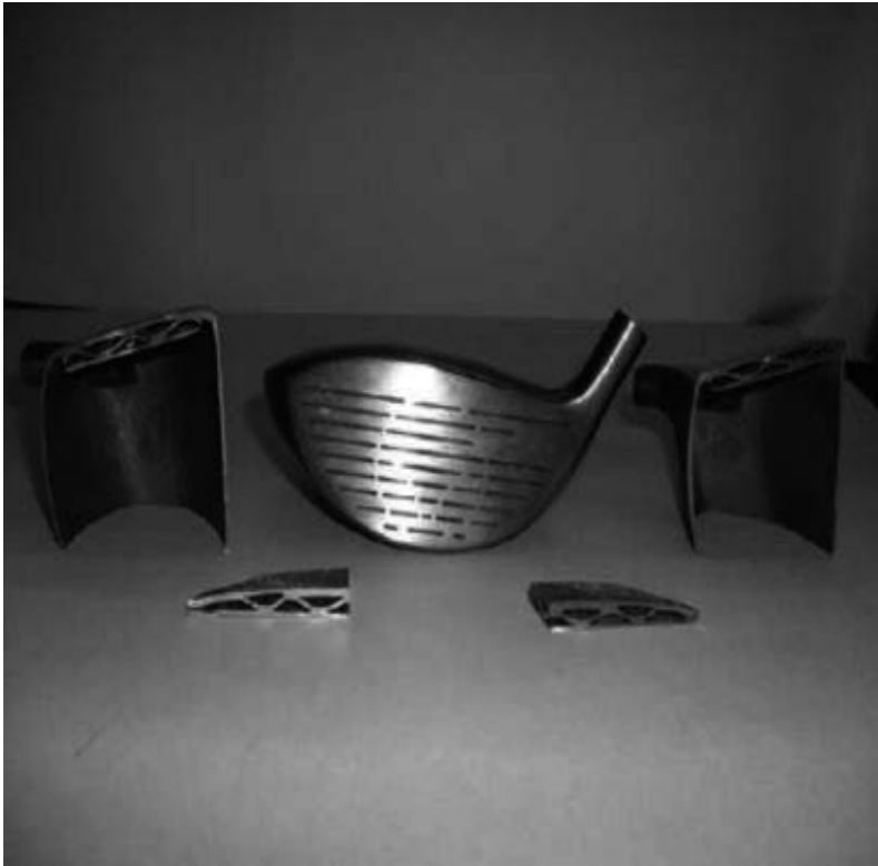
Figure 15. Components of golf club made from nanostructured Ti-6Al-4V alloy [93].
