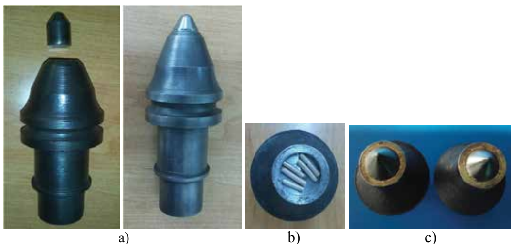
Figure 8. Assemblies prepared for brazing: (a) as-cast steel body and tungsten carbide tip; (b) solder wire placed in the brazing gap; (c) brazed assemblies [3, 7].
