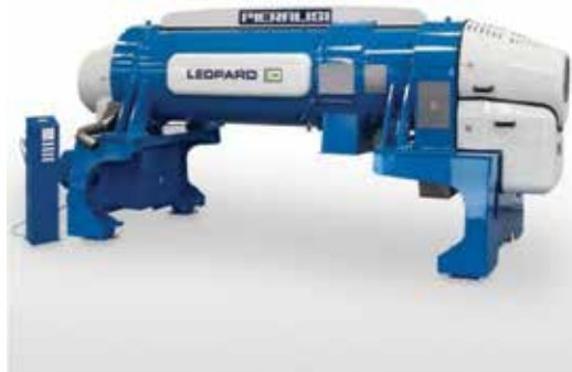
Figure 8. Last generation decanter extractors of olive oil, which combines the two-phase extraction technology without the addition of water with batch processing, thanks to the bowl discharging device. The installed power ranges from 7.5 Kw (more adapted to small quantities of olives to be extracted, i.e. process capacity of 0.5 tonnes/hour) to 45 Kw (for very large quantities of olives to be extracted, i.e. process capacity of 9 tonnes/hour) (Source: courtesy of Perialisi SpA, Ancona, Italy).
