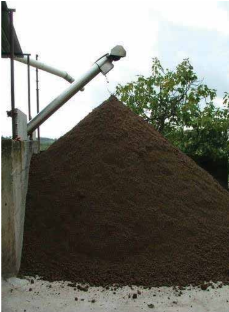
Figure 2. Olive pomace (wet husks) from the two-phase decanter centrifugation olive oil extraction. The wet husks have an initial relative humidity of 65–70% (Source: Marco Nuti).
