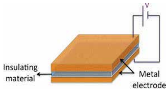
Figure 1. Schematic and electrical configuration of a two-terminal RRAM cell.
