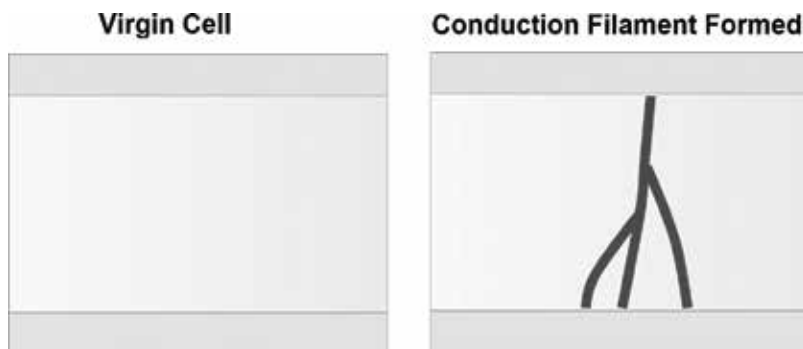
Figure 5. Left: virgin cell. Right: Cell with conduction filament formed.
