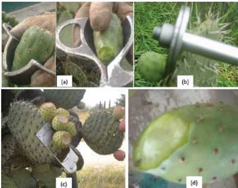
Figure 4. Device (a) slicing the pear straight, (b) electrically driven, (c) cutting with a simple knife, (d) slicing the fruit poorly.
