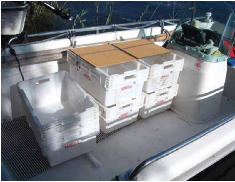
Figure 5. CrayShower on board transport application. This system uses lake surface water, thus not suitable during warmest summer days.
