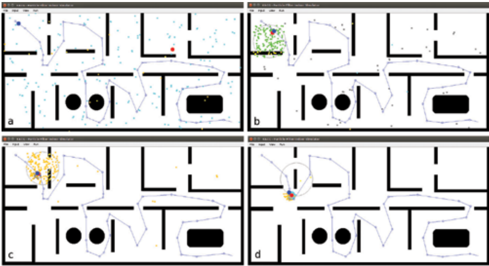
Figure 4. Particle filter in action: 100 particles were randomly located in the building (a), a WiFi positioning service was used for fast converges (b and c). All the particles converged to the correct position (d).
