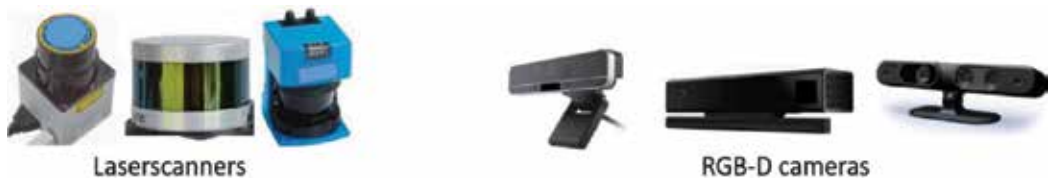
Figure 1. Sensors commonly used in mobile robotics for perception systems.
