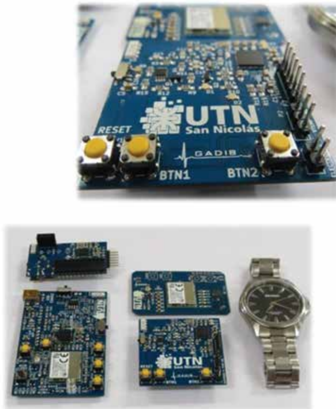
Figure 2. Wearable modules. Up: master module. Down: slaves modules for heart rate/SpO 2 , IMU, temperature, and microphone. It is important to note the size related with a wristwatch.
