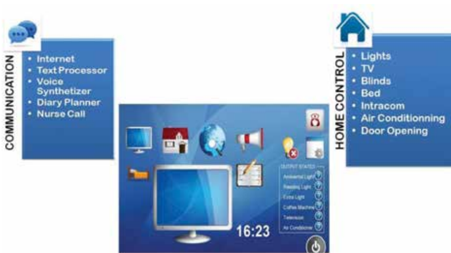
Figure 4. Principal panel of SICAA system and submenus with functions for communication and for home control. The icons, colors, and size were designed especially for people with poor contact with technology.
