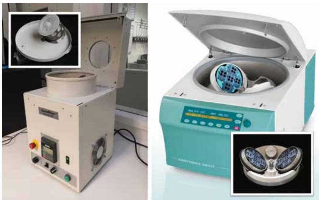
Figure 8. Pictures of the two dual centrifuges: the Speedmixer DAC 150 FVZ (left) and the ZentriMix 380 R (right). Their respective rotors with typical vial holders are shown in the small pictures.
