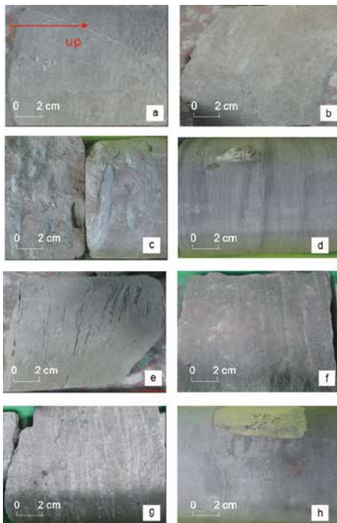
Figure 8. Typical lithofacies of the W79 block for the target interval: (a) parallel bedding sandstone; (b) trough cross-bedding sandstone; (c) scouring structured sandstone with mud gravels; (d) ripple cross-bedding siltstone; (e) wavy cross-bedding siltstone; (f) parallel bedding siltstone; (g) ripple cross-bedding muddy siltstone; (h) flasher structured mudstone (after [19]).
