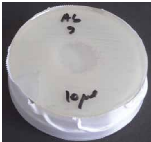
Figure 3. Aromatogram. In the middle of a sterile paper disk, with diameter of a Petri dish lid, 10 µl of essential oil was deposited. After sealing the assembly, the volatile effect was tested.
