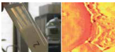
Figure 6. Incompatibility phenomenon in starch paste, AFM image of regular maize starch paste (right, own study, GONOTEC Qscope, USA, non-contact mode).
