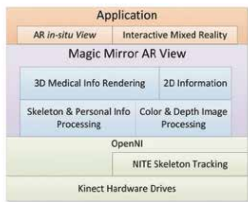
Figure 10. Magic Mirror system framework. The lowest two layers represent the open source library to access the Kinect raw image data and skeleton information. The middle layer is the modules used to create Magic Mirror AR view of the user. The top level is the application with basic system features.
