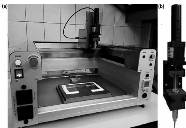
Figure 1. (a) System BioScaffolder, SYSENG and (b) low temperature deposition head.
