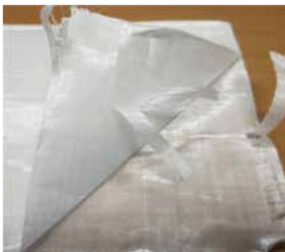
Figure 12. Ballistic panel Spectra Shield® SR-1226 by Honeywell. The sample is delaminated/stratified, showing two panels with two layers each, and the yarns in each panel are positioned perpendicularly; source: author's own photo archives.
