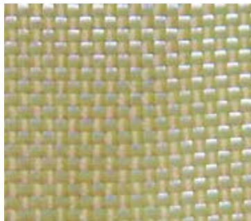
Figure 6. Plain weave fabric made of Kevlar 49® yarns by DuPont; source: author’s own photo archives. Note: Plain weave single fabric; 85 warps/10 cm and 85 wefts/10 cm. Both warps and wefts are made of Kevlar. Total area density: 300 g/m 2 . Thickness: 0.35 mm.
