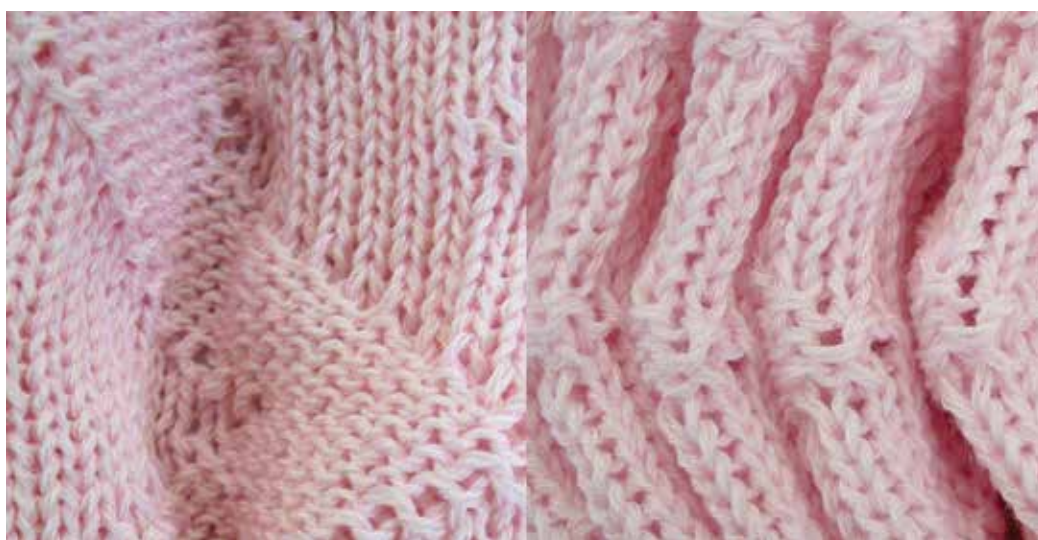
Figure 11. Stiffening folded structure by interlacing additional PA filament (left—no filament, right—incorporated filament).
