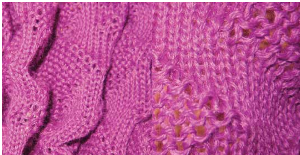
Figure 10. Foldable links-links zigzag structure knitted with different setting of the front and rear cams (left—folded, right—unfolded).
