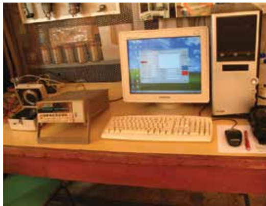
Figure 10. Stand for surface and volume resistivity measurements.
