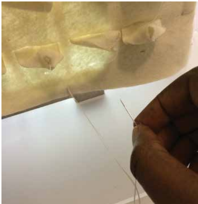
Figure 15. Sewing the felt panel to aluminum frame.
