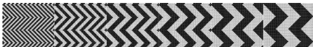
Figure 8. Pattern chart of zigzag knitted structures with different widths of zigzag line (size of repeating unit cell from left to right: 4 \times 24 , 8 \times 24 , 12 \times 24 , 16 \times 24 , 20 \times 24 and 24 \times 24 ).
