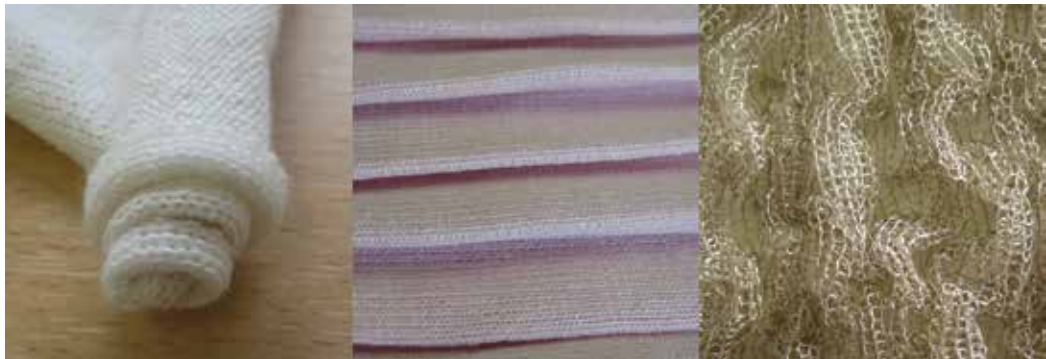
Figure 4. Foldable knitted structures: roll, pleats, bubbles.
