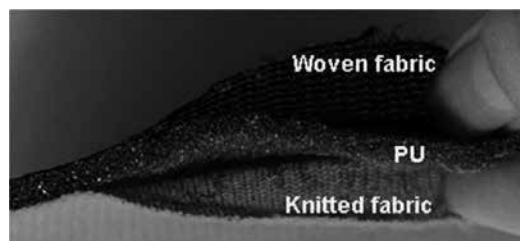
Figure 3. Composite material for car seat upholstery.
