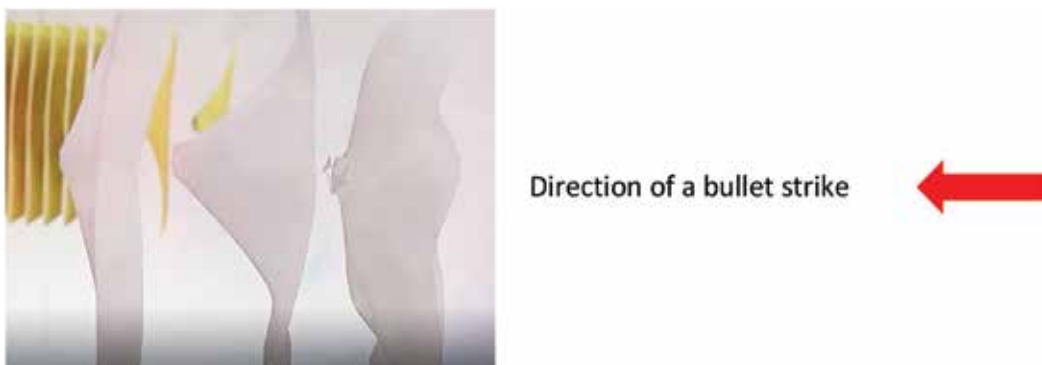
Figure 15. Characteristic cone shapes in the layers of a soft protective panel elements after the bullet struck and perforated them, heading in the direction of the next layer. The cones become smaller due to the smaller amount of bullet kinetic energy transferred to each consecutive layer; prepared on the basis of a Tensylon™ commercial released by DuPont.
