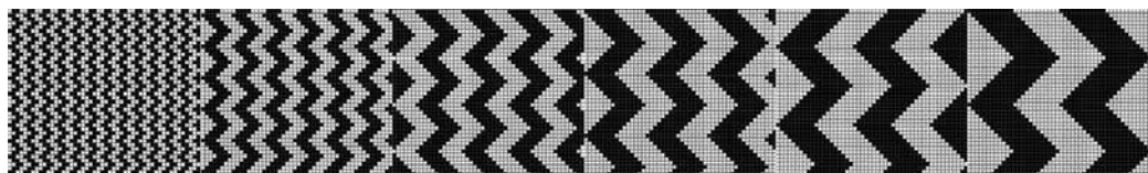
Figure 6. Pattern chart of zigzag knitted structures with different square repeating unit cell sizes (size of repeating unit cell from left to right: 4 \times 4 , 8 \times 8 , 12 \times 12 , 16 \times 16 , 20 \times 20 and 24 \times 24 ).
