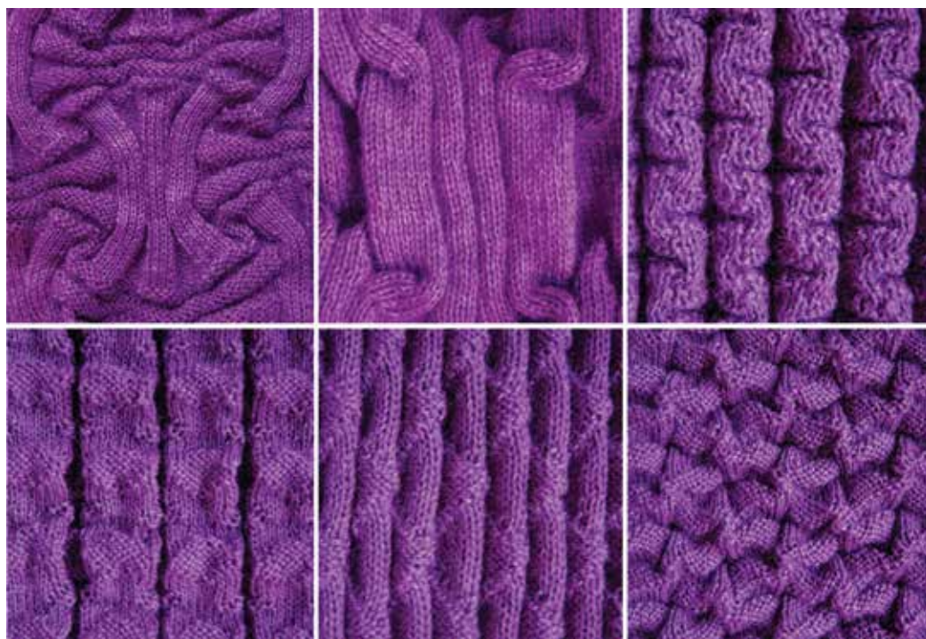
Figure 5. Various foldable links-links knitted structures.
