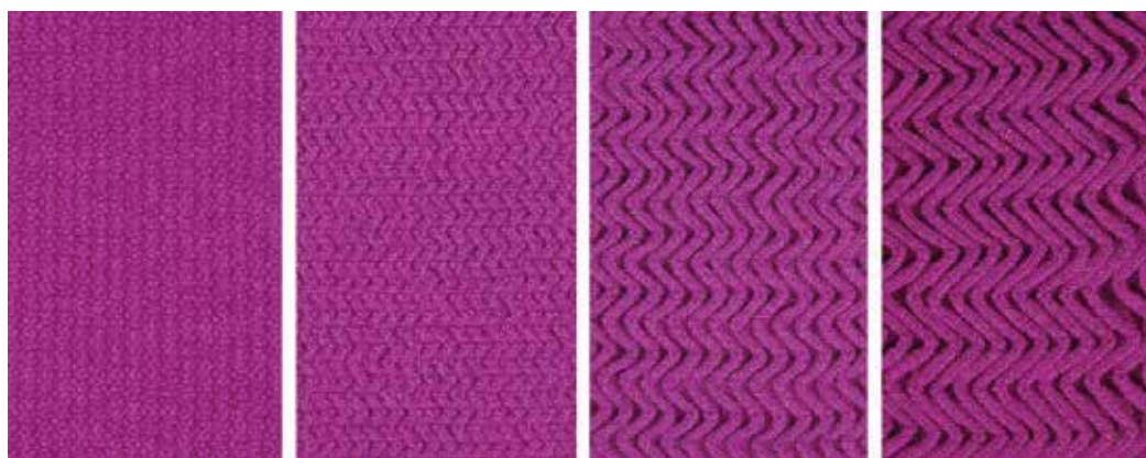
Figure 7. Zigzag knitted structures with different square repeating unit cell sizes made of WO/PAN yarn (size of repeating unit cell from left to right: 4 \times 4 , 8 \times 8 , 16 \times 16 and 24 \times 24 ).
