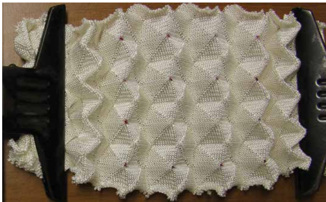
Figure 13. Measuring dimensional changes for evaluating auxetic potential.
