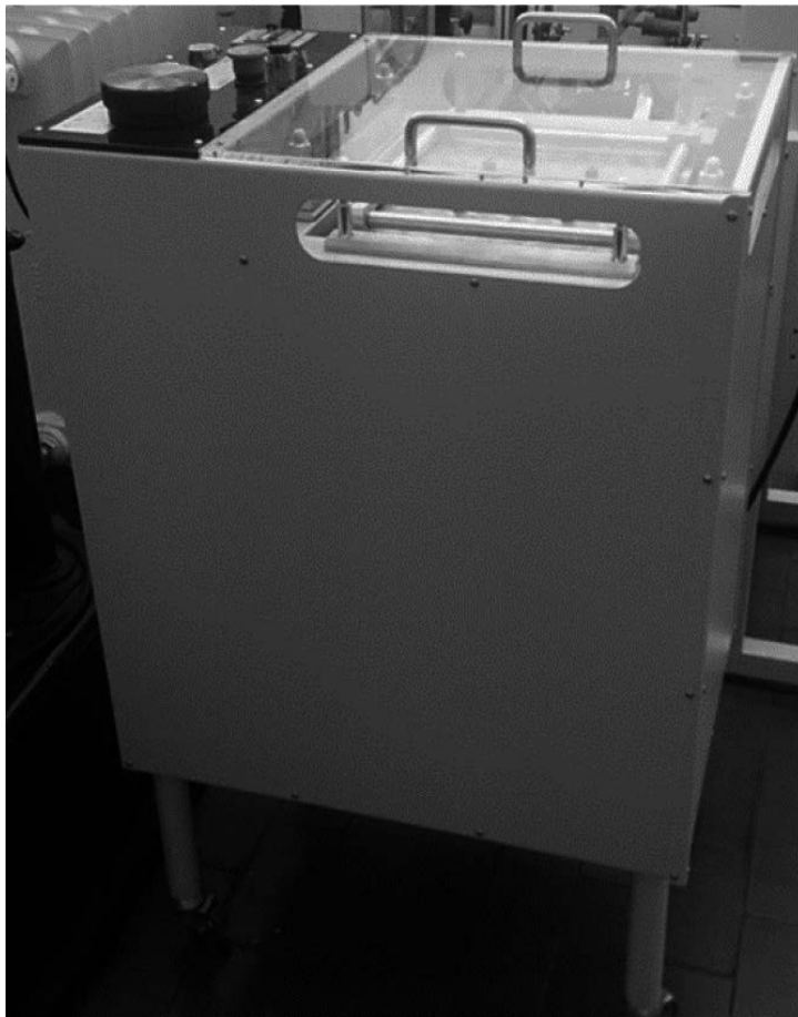
Figure 12. The device for measuring uniaxial and biaxial cyclic stress.
