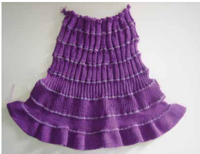
Figure 3. Folding of ribbed structures with various rib widths made on the same number of knitting needles.
