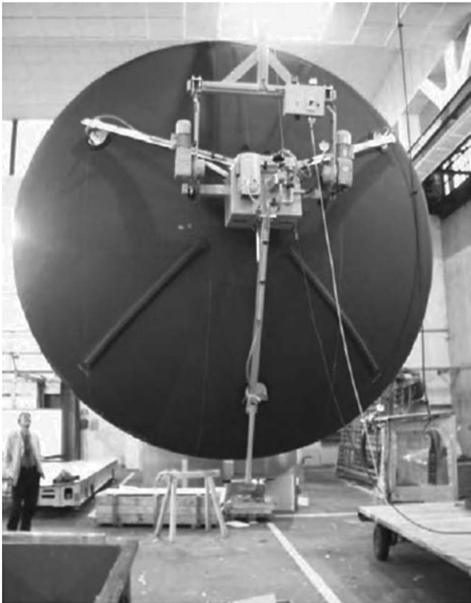
Figure 11. Rear pressure bulkhead of the Airbus A380 [90].
