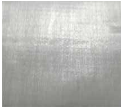
Figure 13. Ballistic panel Spectra Shield® II SA-4144 panel by Honeywell; source: author's own photo archives. Note: From a distance, Spectra Shield® II SA-4144 is difficult to distinguish from Spectra Shield® SR-1226. The organoleptic assessment of the samples allows an easy verification. Spectra Shield® SR-1226 is thicker, stiffer and has a more waxy tactile sensation.
