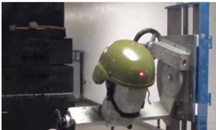
Figure 25. A ballistic test set up for testing a MICH ballistic helmet against 9 mm calibre; source: www.kick-az.com .
