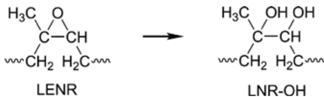
Figure 12. Schematic diagram representing reaction of ELNR to LNR-OH [86].
