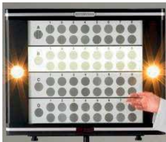
Figure 4. CSV-1000E used for glare testing at varying luminance and contrast sensitivity at different spatial frequencies. Image courtesy of VectorVision [40].
