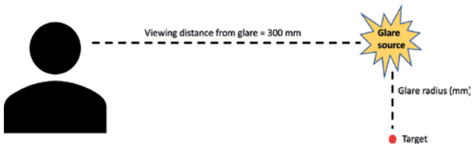
Figure 5. Schematic of the Halometer glare device utilized by Babizhayev and colleagues to measure intraocular light scatter in subjects with cataracts. Babizhayev et al. [45].
