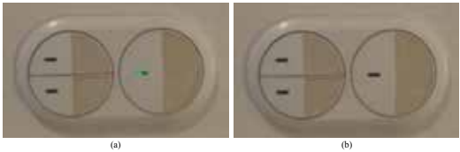
Figure 17. Push-type switch. (a) ON; (b) OFF.
