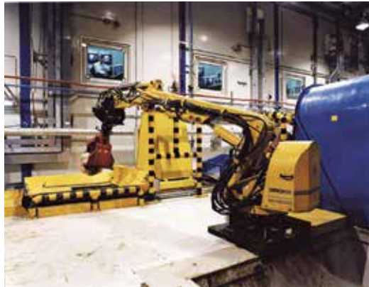
Figure 1. A BROKK robot, equipped with a gripper, being used for a pick and place task at the Sellafield nuclear site in UK. Human operator can be seen controlling the robot from behind a 1.6m thick lead-glass window which shields him from radiation, but significantly limits his situational awareness. For more examples, refer to www.sellafieldsites.com/solution/decommissioning .
