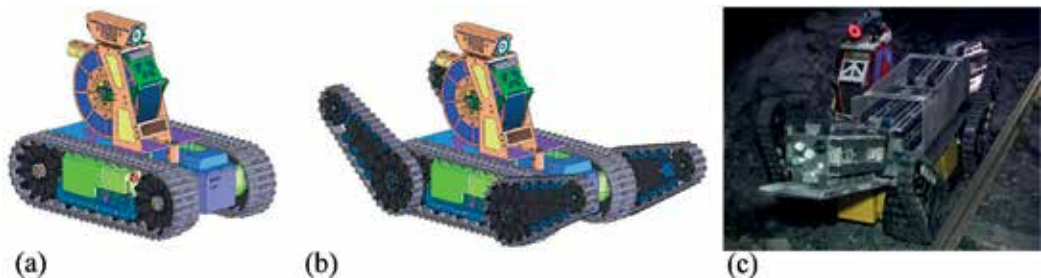
Figure 1. Modular structure of MINBOT-II. (a) Robot without arms; (b) Robot with front and back arms; (c) Actual coal mine robot.
