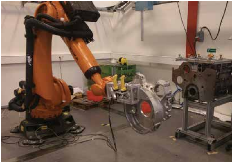
Figure 1. Enabling device for hand-guiding, the ToMM project (handles on the gripper).
