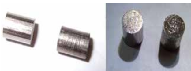
Figure 6. Pd-rod specimen before and after irradiation (one can see it layered structure) and black surface view, which was close to SNO.
