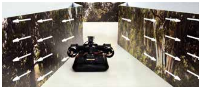
Figure 2. The LORA robot fitted with a heading-lock system travels straightforward through a tapered corridor perceiving a purely translational optic flow. This optic flow experienced by the robot is schematized by the white arrows (i.e., angular velocity vectors) on the walls (adapted from [25] under CC-BY license).
