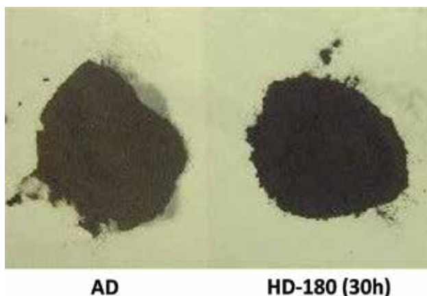
Figure 13. Color differences between two samples of finely ground sewage sludge. AD: air-drying, HD-180 (30h): heat-drying at 180°C with a stabilization period of 30 hours.
