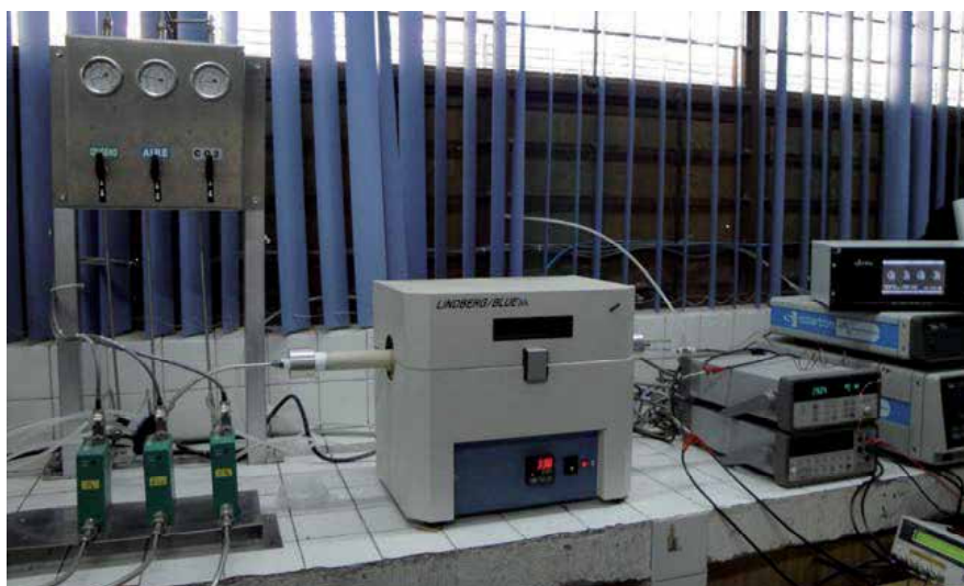
Fig. 4. Image of the instruments used for the gas sensing measurements.
