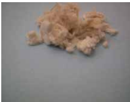
Figure 10. Cellulose fiber obtained from esparto grass.
