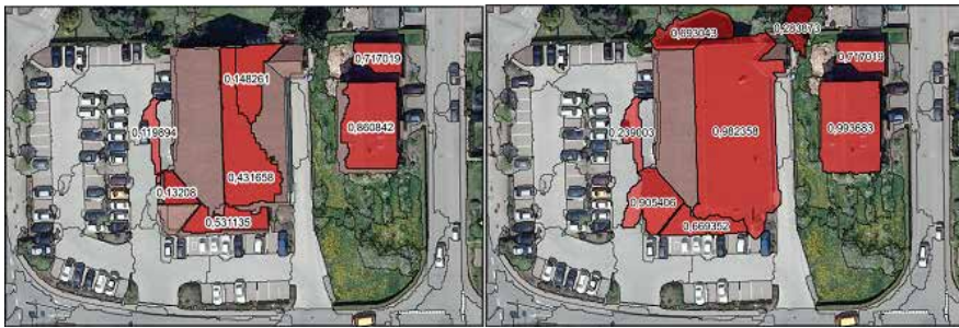
Figure 5. Segmentation and classification result before (left) and after (right) applying the agent-based optimization approach according to the ABIA framework. Numbers indicate the membership degree to “building” (Source: [38]).
