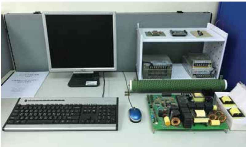
Figure 6. Photo and parameters of a PSPWM full-bridge power converter circuit. Transformer turns ratio n = 0.5 . V_i = 160 volt, V_0 = 50 volt, R = 6\Omega , C = 940\mu F , L = 300\mu H , L_{lk} = 20\mu H , C_A = C_B = C_C = C_D = 5nF , f_s = 50 kHz.
