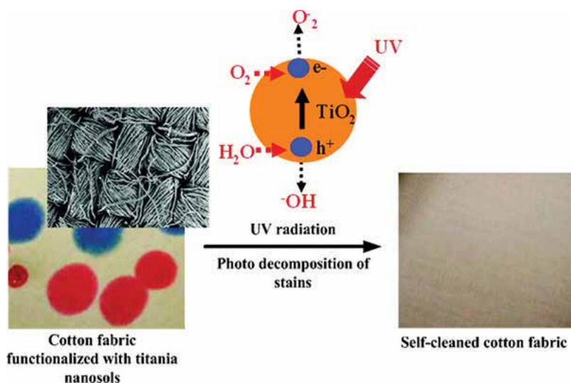
Figure 8. Self-cleaning properties of cotton fabric treated with titania nanosols. Copyright 2009 American Chemical Society [45].
