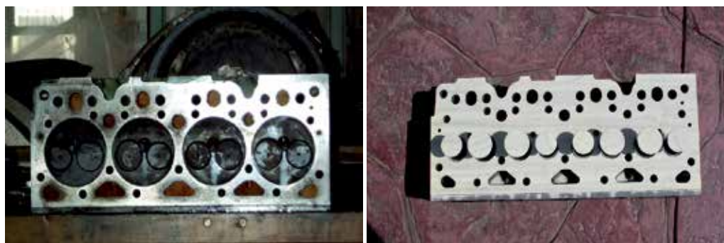
a) Cylinder heads and valves without coating b) Ceramic coated cylinder heads and valves Fig. 11. Cylinder head and valves before coating and after coating
