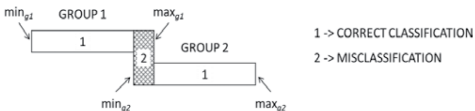
Figure 3. Procedure for selecting appropriate acoustic features. The value of 1 indicates correct classification, and the value of 2 indicates incorrect classification. Parameters " max_{g1} " and " min_{g2} " indicate maximum and minimum threshold limits for incorrect classification.
