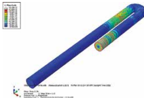
Figure 6. Displacement magnitude after propagation of a 10-cycle 40 kHz pulse around the bend.
