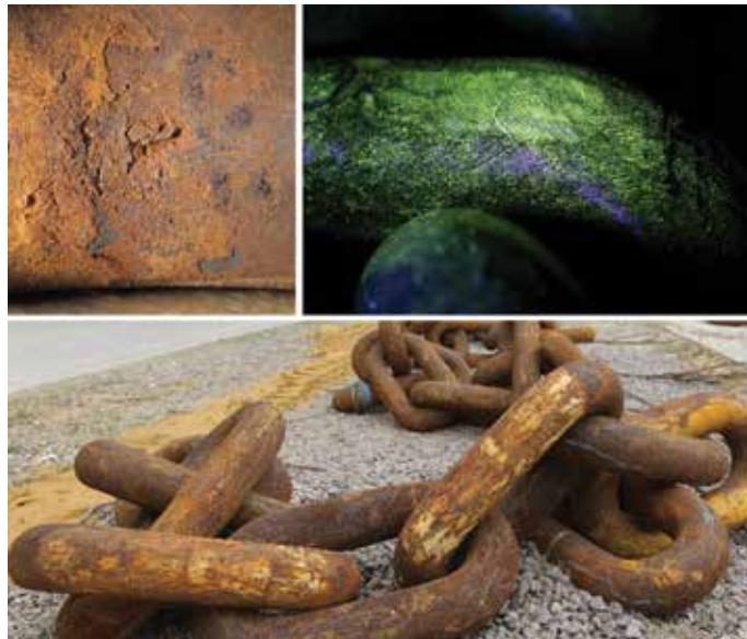
Figure 1. From left to right: Example of wear and corrosion on a chain link from the sea-bed touch down zone, in-water inspection showing a studded chain which has lost its stud in situ , illustration of marine growth on long-term deployed chain, affecting optical in-water inspection, friction-induced bending.
