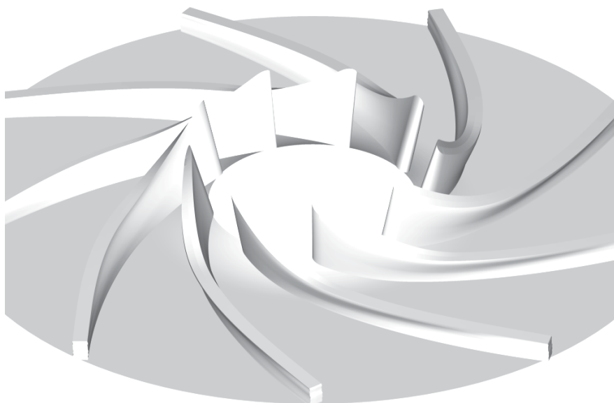
Fig. 32. 3D image of the rear shroud with blades (front shroud disk was removed)
