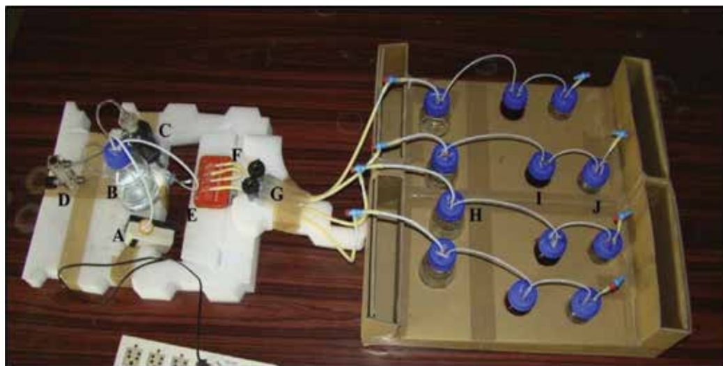
Figure 2. Microcosm system constructed in the laboratory [23]. Air pump (A), 2 M NaOH (B), activated charcoal (C), rotameter (D), 0.2 \mu cellulose acetate filter (E), glass manifold (F), air regulator (G), sterile MilliQ water bottle to maintain humidity (H), microcosm flask (I) and CO 2 trap (J).
