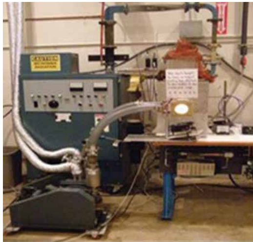
Figure 9. High-temperature microwave plasma furnace used for nitrogen plasma passivation (N-plasma passivation).
