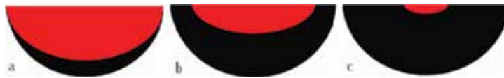
Figure 14. Schematic diagram of the solidification process of silicon cake: (a) the initial stage, (b) the intermediate stage and (c) the end stage.
