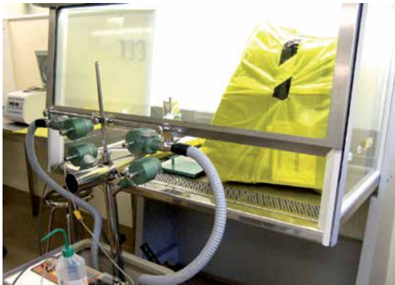
Fig. 2. The unique potassium iodide KI-discus-test, to validate a class II safety cabinet with a DNA isolation robot in a BSL-3 laboratory. The KI discus test is defined in the European Standard for microbiological safety cabinets, EN12469:2000 as a test method for validating the operator protection capabilities of the cabinet (Photo: SVA).
