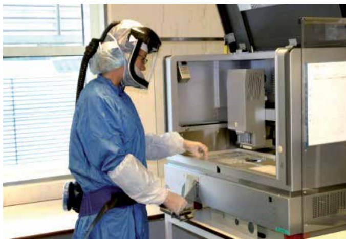
Fig. 3. Up-scaling capabilities by the use of automated DNA extractions robot in a BSL-3 laboratory (Photo: SVA).
