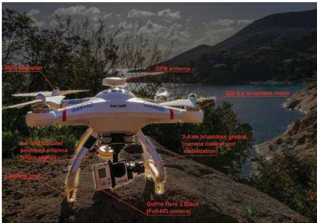
Figure 1. The Quantum Nova CX-20 Quadcopter ready to fly just before a coastal mapping mission.
