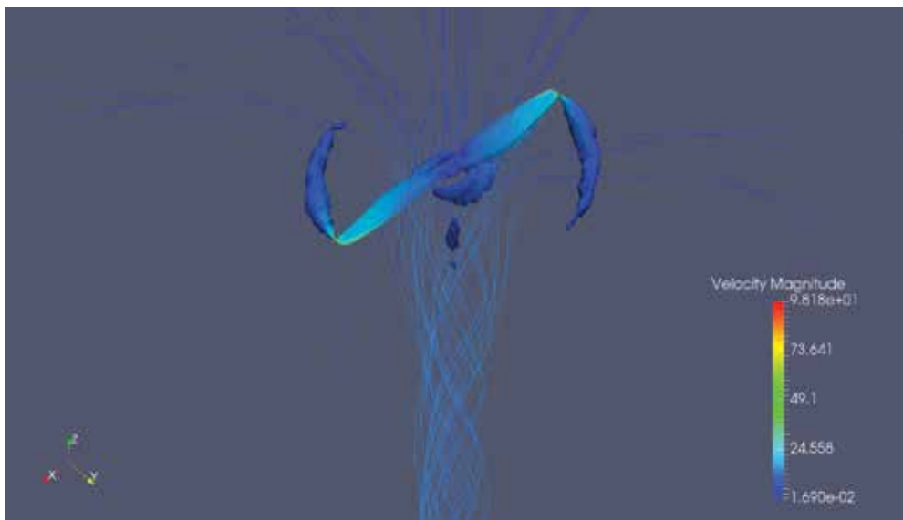
Figure 9. Streamlines colored by velocity magnitude and contours of Q -criterion = 50,000, at 4500 rpm.
