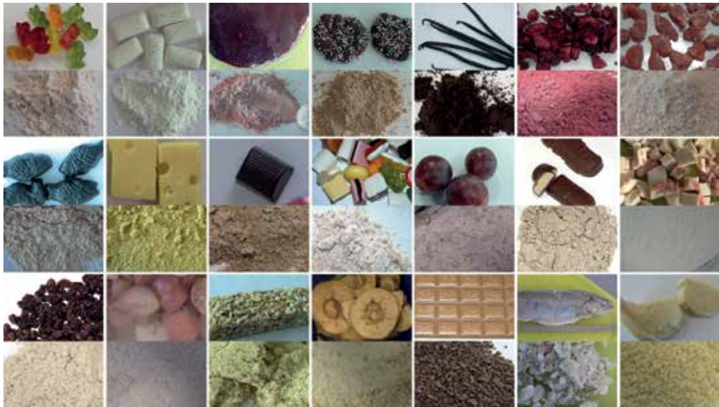
Figure 16. Food samples ground under cryogenic conditions; first row from left to right: jelly bears, chewing gum, fresh liver, cookies, vanilla pods, dried cherries, fresh meat; second row from left to right: licorice, cheese, praline with liquid core, wine gum, grapes, block of marzipan, bacon; third row from left to right: raisins, onions, bar of cereals, dried apples, block of chocolate (pre-ground), frozen fish (pre-ground), cocoa butter (pre-ground).
