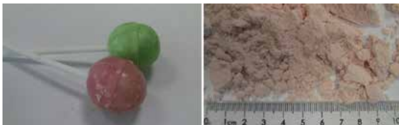
Figure 13. Homogenization of candy; left to right: original sample, sample ground to <500 \mu\text{m} .
