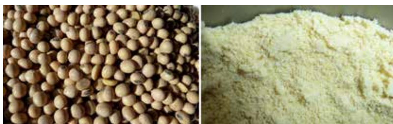
Figure 14. Homogenization of soy beans; left to right: original sample, sample ground to <500 \mu\text{m} .
