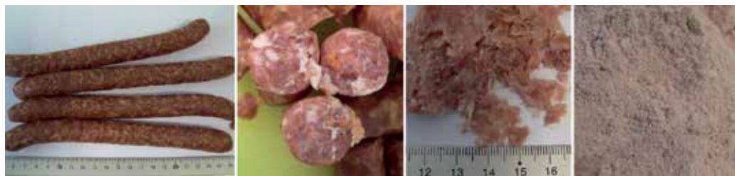
Figure 5. Homogenization of sausages; from left to right: original sample; pre-cut sample with large fatty parts; sample ground to <5 \text{ mm} ; pulverized sample of <300 \mu\text{m} .
