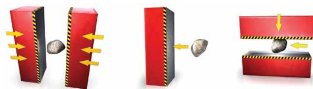
Figure 3. Size reduction principles for hard and brittle materials: pressure, impact, and friction.
