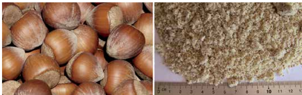
Figure 7. Homogenization of nuts; from left to right: original sample; pulverized sample of <math><300 \mu\text{m}</math>.
