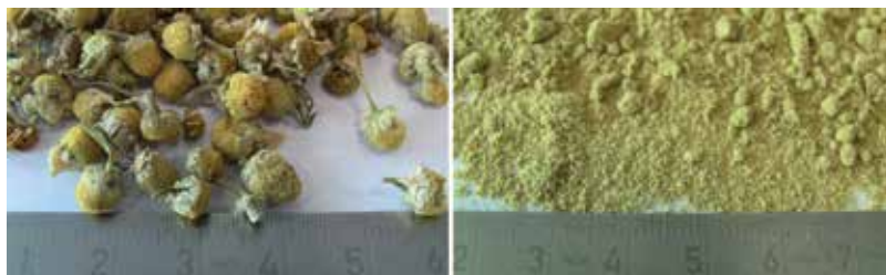
Figure 10. Homogenization of chamomile; left to right: original sample, sample ground to <100 \mu\text{m} .
