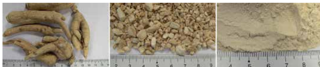
Figure 11. Homogenization of ginseng; left to right: original sample, sample ground to <8 \text{ mm} , sample ground to <100 \mu\text{m} .
