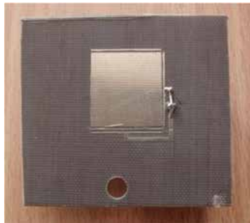
Figure 2. Photograph of fabricated microstrip T-stub coupled patch antenna.
