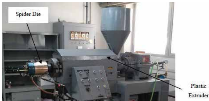
Figure 10. Johnson Plastics single-screw extruder together with the mounted extrusion die.
