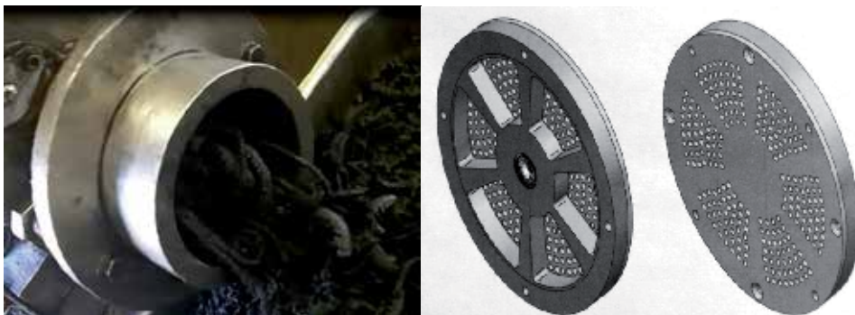
Figure 4. Shearing through the shearing plate extruder; view of shearing plate.
