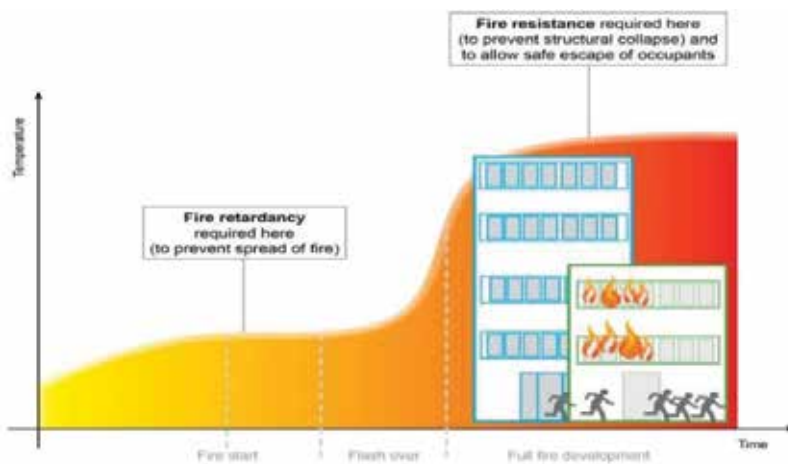
Figure 1. Phases of fire development in an enclosure.
