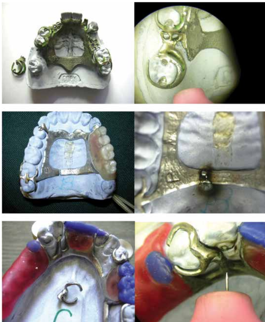
Figure 16. Some fractured metallic frameworks of removable partial dentures, before and after welding.
