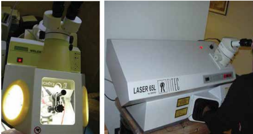
Figure 20. The micro pulse welding device Welder (Schütz dental) and laser 65 L-Titec with welding parameters.
