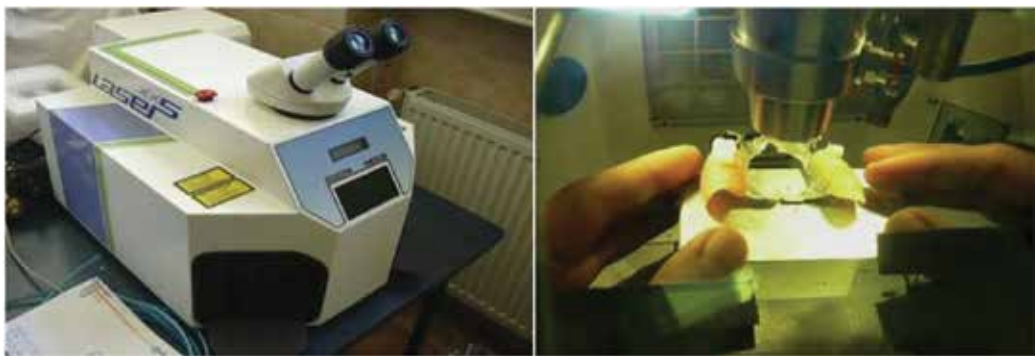
Figure 4. XXS laser welder for dentistry (Orotig) and its enlargement system.
