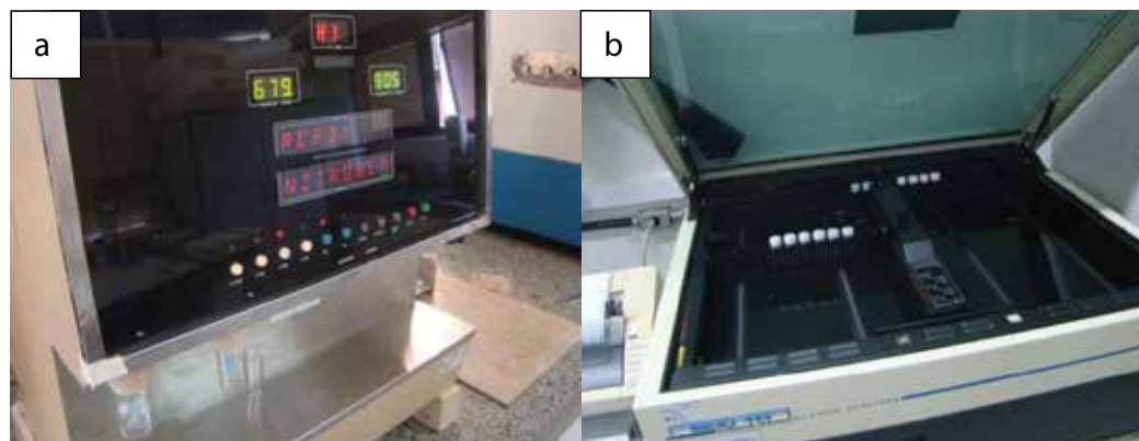
Figure 3. Oxidizer OX500 (R.J. Harvey Instrument Corporation) (a) and liquid scintillation equipment, Tri-Carb 2910 TR LSA counter (PerkinElmer) (b) from the Laboratory of Ecotoxicology of CENA/USP.
