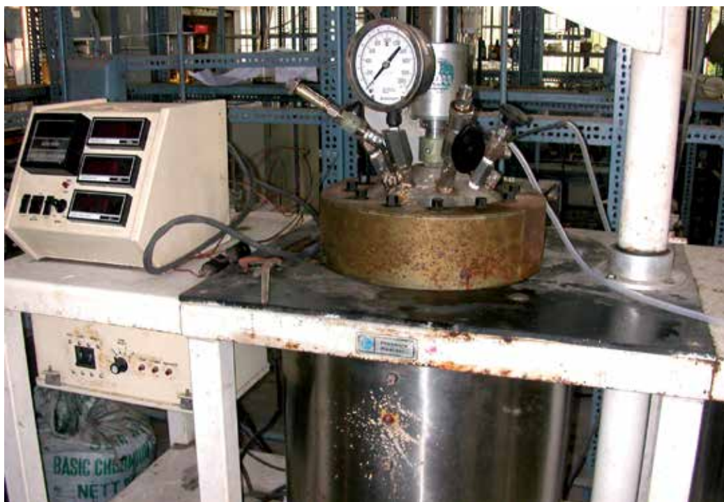
Fig. 3. Bench Scale lab Parr Reactor
