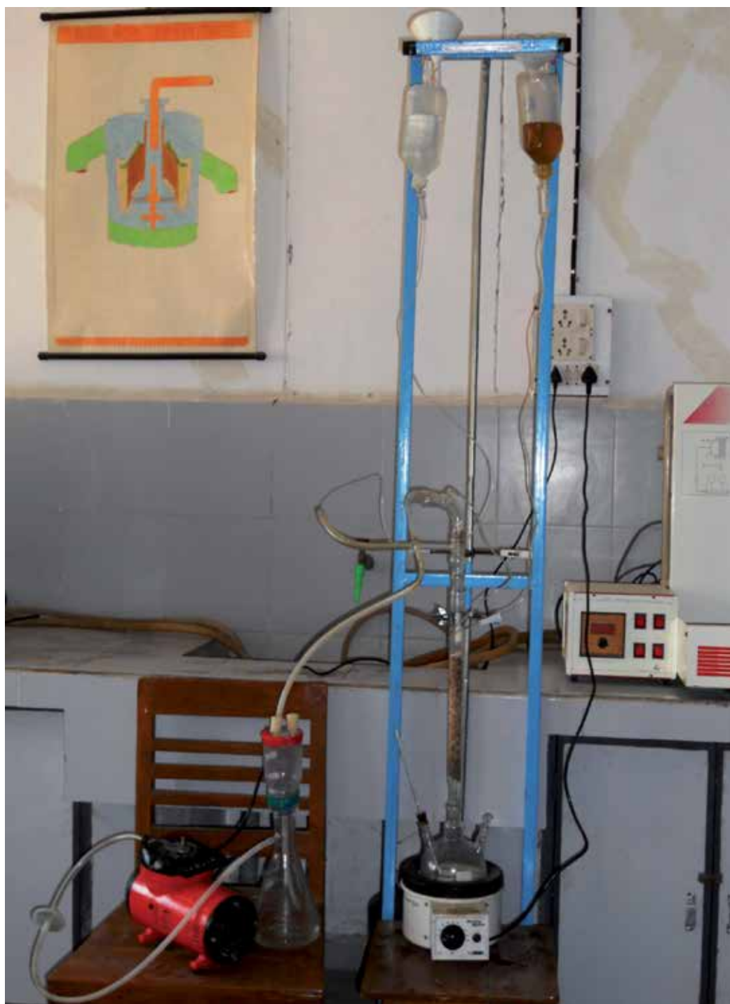
Fig. 7. a) View of experimental lab apparatus of Reactive distillation
