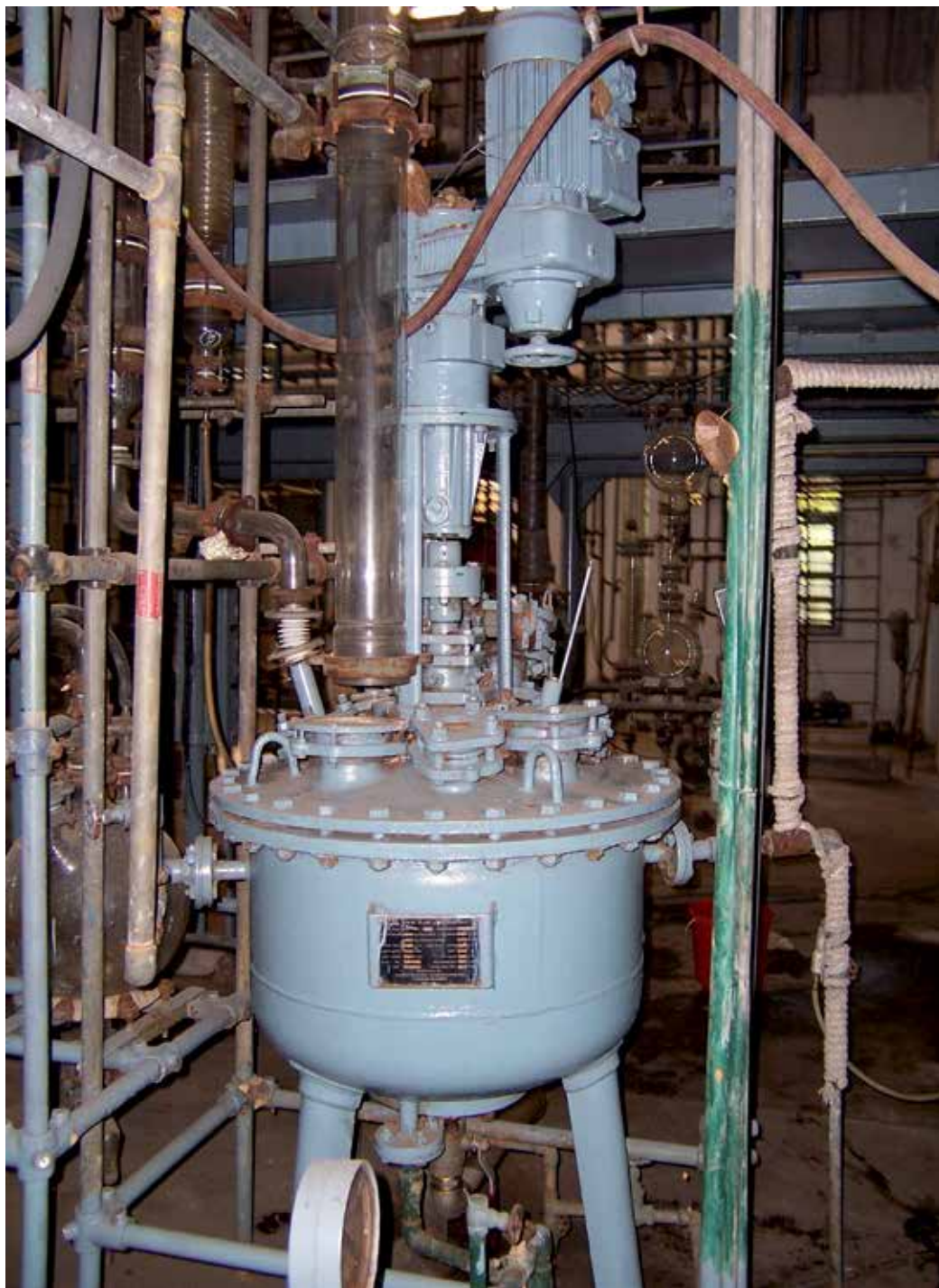
Fig. 5. (b) Pilot Plant scale reactor
