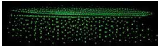
Figure 15. Video image of light scattered by spherical divinylbenzene particles of 2.74 \pm 0.09 \mu\text{m} in diameter suspended in argon plasma at 65 Pa.
