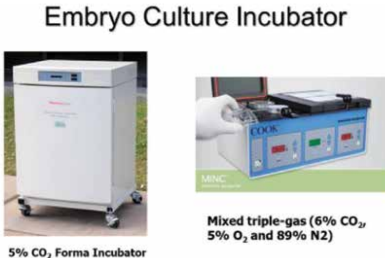
Figure 1. Embryo culture incubators. Two kinds of incubators are shown as big-box incubator (left) and Cook Bench Minc incubator (right).
