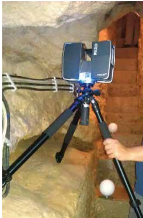
Figure 4. A TLS station positioned as close, as possible to the cave wall to “see” into a vertical chimney. The white spheres are the artificial backsight targets kept in position till the next session is measured from a subsequent station.
