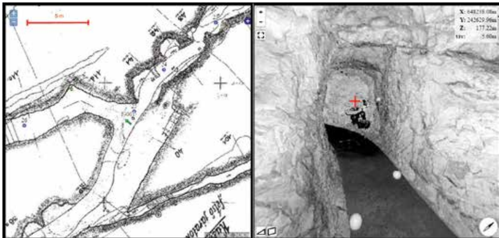
Figure 5. Archive map (left) and TLS survey image (right) in a common reference system. The map is oriented to the North. Green arrow indicates the position of the TLS station pointing toward the line of sight of the intensity image shown in the right panel. Geodetic coordinates of the station and the cursor position is displayed. The figure is created with a web viewer, which was designed to explore the TLS data beforehand thorough data processing [20].
