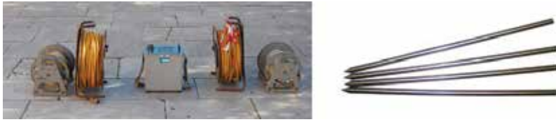
Figure 2. Resistivity equipment: left, automated resistivity metre and cables; right, stainless steel electrodes.
