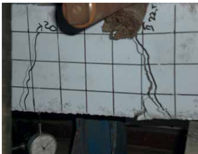
Figure 8. The crack pattern of the bamboo reinforced concrete beam after being tested [22].
