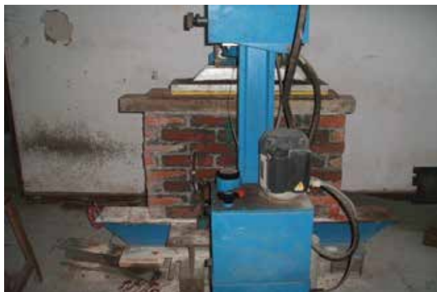
Figure 1. The brick masonry compressive strength test.
