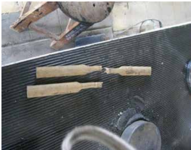
Figure 7. The bamboo was tested until it was Fracture [21].
