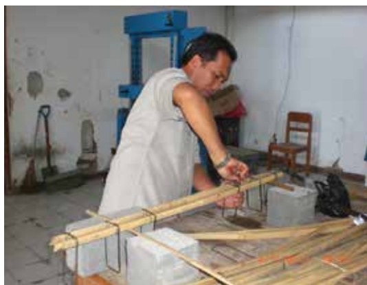
Figure 3. The bamboo reinforced concrete beam assembled was 120 mm × 250 mm. The reinforcement area were 400 and 1200 mm 2 [22].
