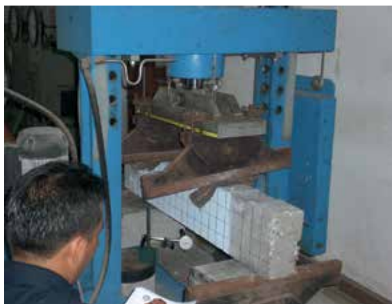
Figure 4. The loading test of concrete beam which 120 mm × 250 mm with the reinforcement area were 400 and 1200 mm 2 [22].
