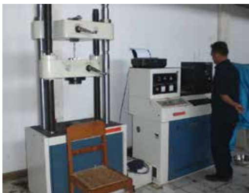
Figure 2. Standard machine used to test the bamboo tensile strength [22].
