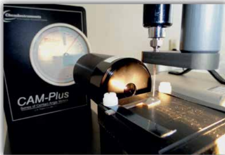
Figure 5. Experimental setup for contact angle measurement.
