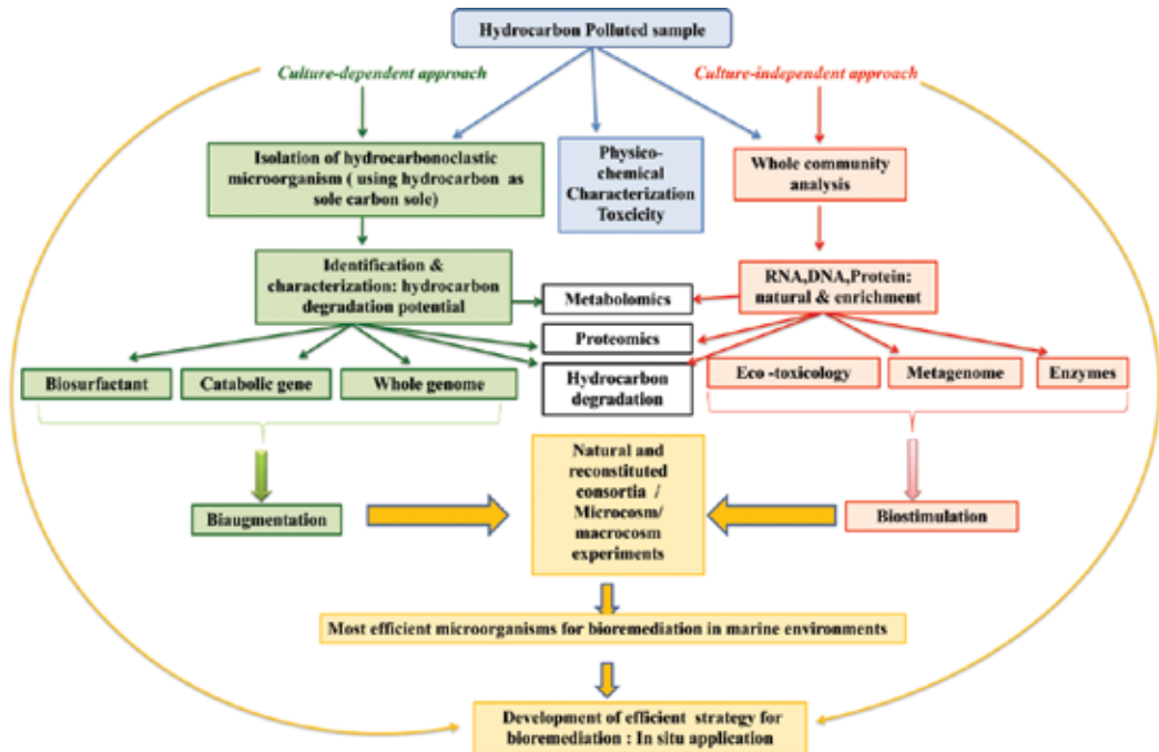
Figure 5. Schematic diagram explaining the different microbial hydrocarbon degradation strategy for bioremediation.
