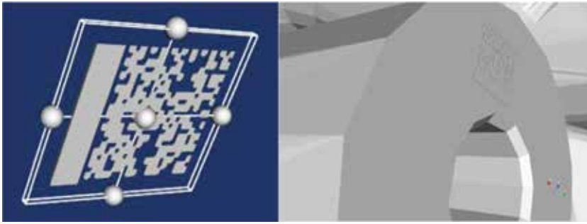
Figure 9. Using an STL model to define the robot task.
