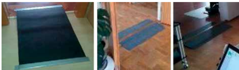
Figure 3. Several examples of mats and ramps to make the floor flat enough for a wheeled robot.
