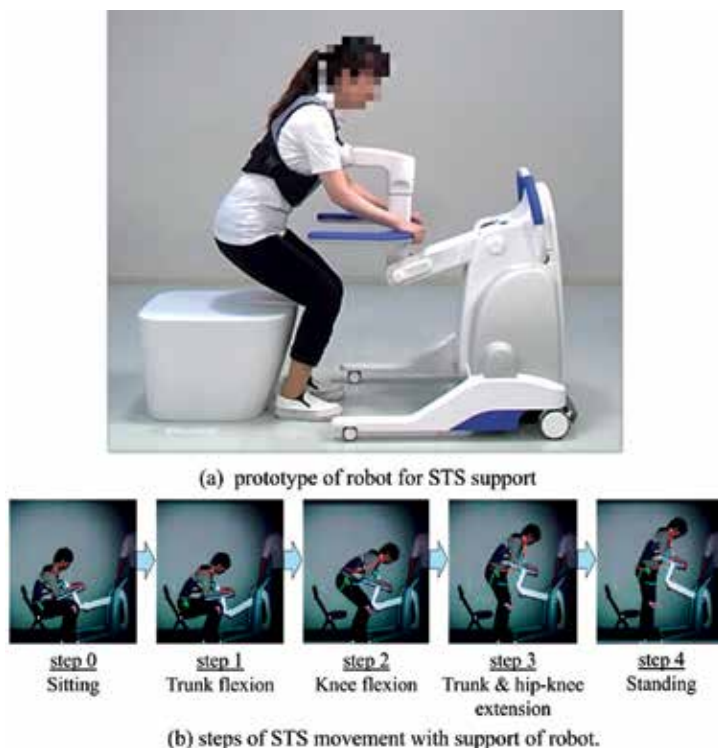
Figure 2. Overview of service robot. (a) A prototype service robot, complying with the ISO/TS 15066:2015 standard, with end-effect forces of 240 and 100 N in horizontal and vertical directions, respectively; (b) steps in robot-assisted STS movement, step (0) sitting still; step (1) trunk flexion; step (2) knee flexion; step (3) trunk and hip-knee extension; step (4) stabilization.
