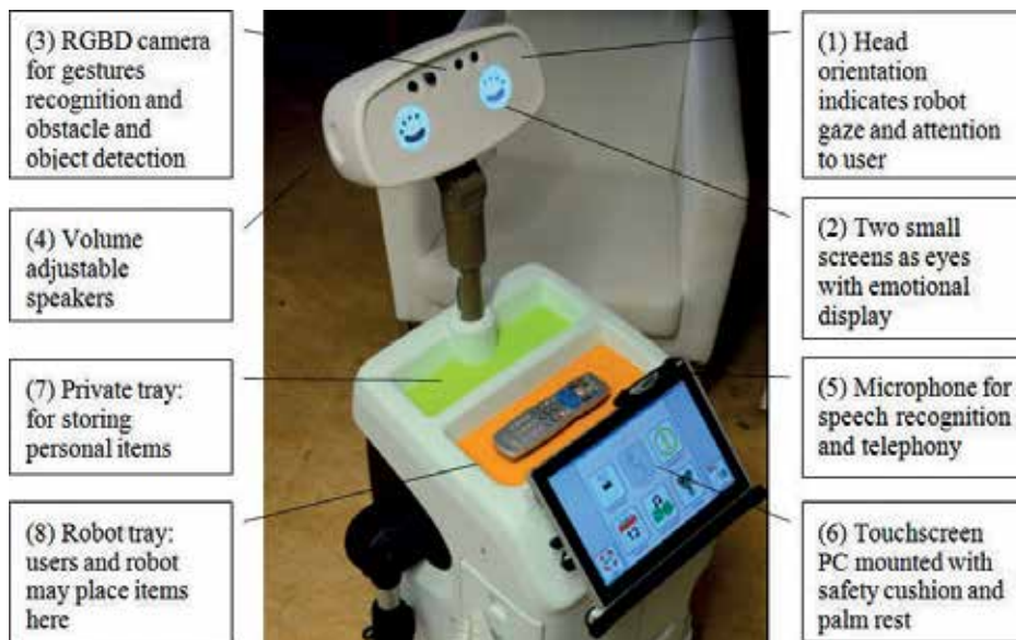
Figure 7. The upper body and the head of Hobbit. Also, depicted are the main components and functionalities.
