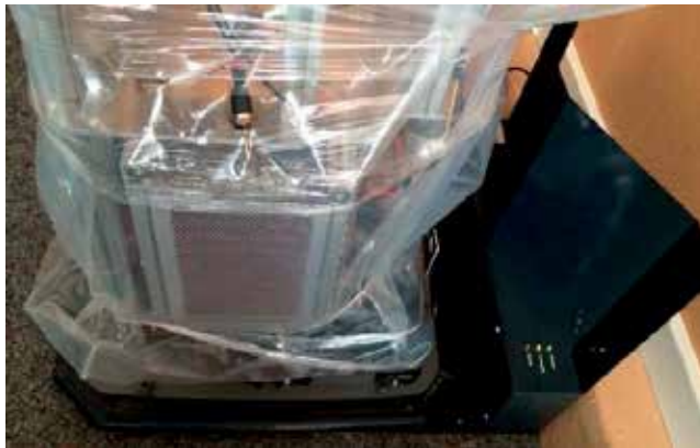
Figure 4. Docking station (black) and the robot wrapped in plastic for temperature tests.
