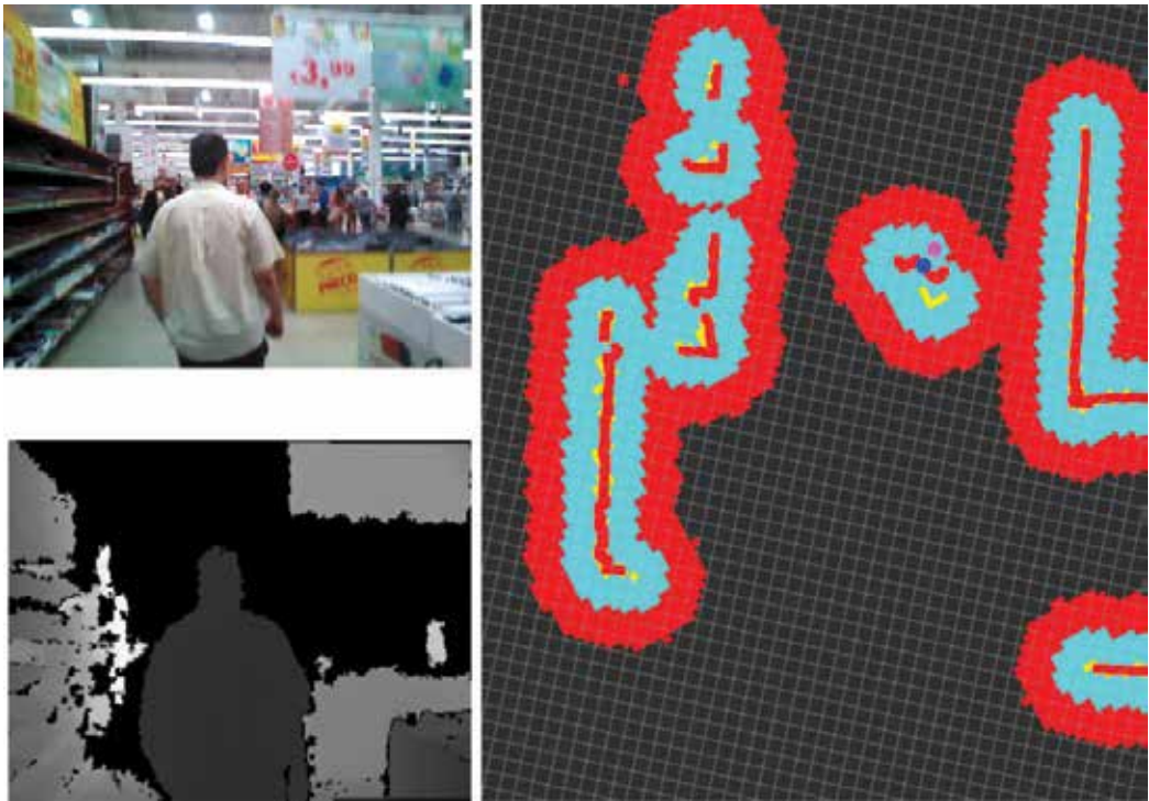
Figure 8. Tracking example where the person is visible both by the vision and by the 270° laser scanner. Purple dot in the map image corresponds to the person as localized by the image module, while the blue dot corresponds to the person as localized by the 270° laser scanner.
