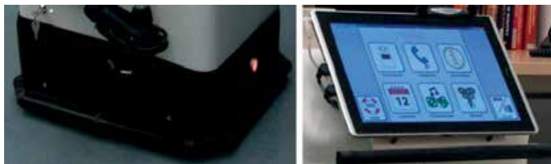
Figure 5. Safety bumper all around the base plate (left, only the front view of the robot is shown) and (right) tablet base bumper (the black rubber band below the tablet).
