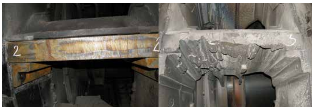
Figure 2. New grinding table (left) and worn grinding table (right).
