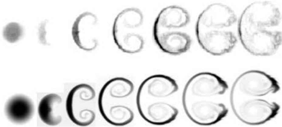
Figure 9. Evolutions of SF 6 gas cylinder, upper row corresponding to experiment, lower row corresponding to numerical simulation by MVFT program, the time sequences are 0, 50, 190, 330, 470, 610, and 750 μs severally.
