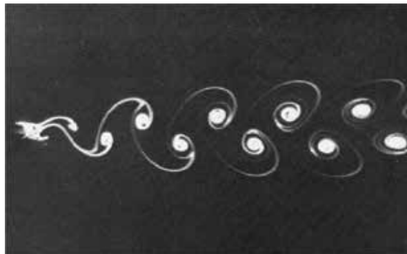
Figure 2. Von Karman streets behind a cylinder in a nonrotating 2D flow for Re = 140 , fluorescein visualization, picture taken from [3].
