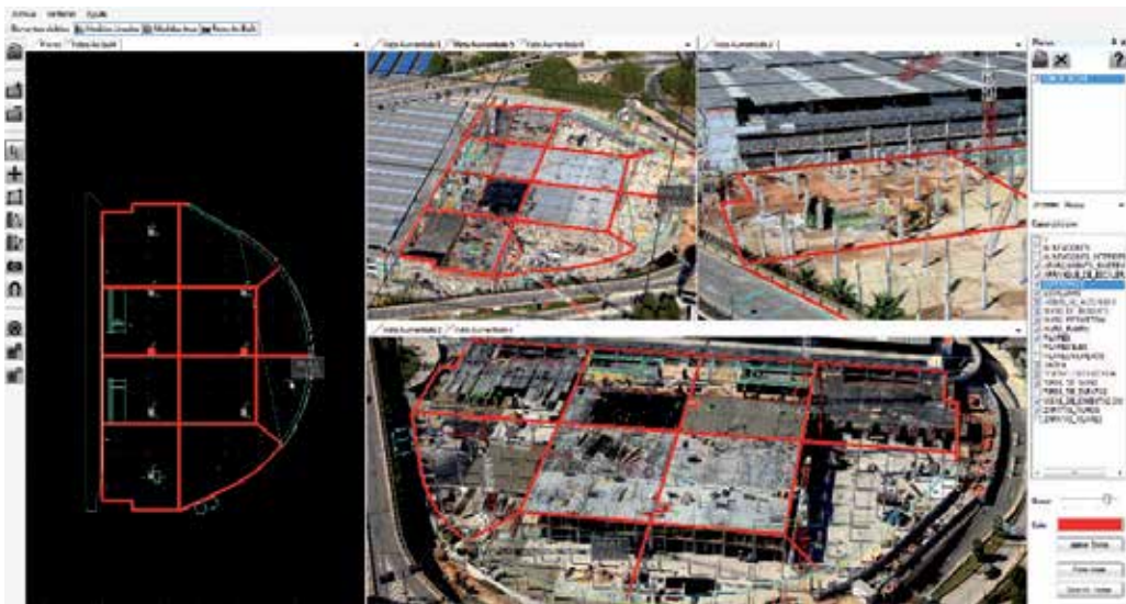
Fig. 11. Image of the system in the construction of a parking area using aerial images as background for the augmented views.
