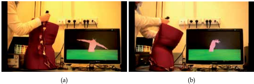
Fig. 18. (a) Lateral and (b) front measured trunk movements are replicated on a pc screen.
