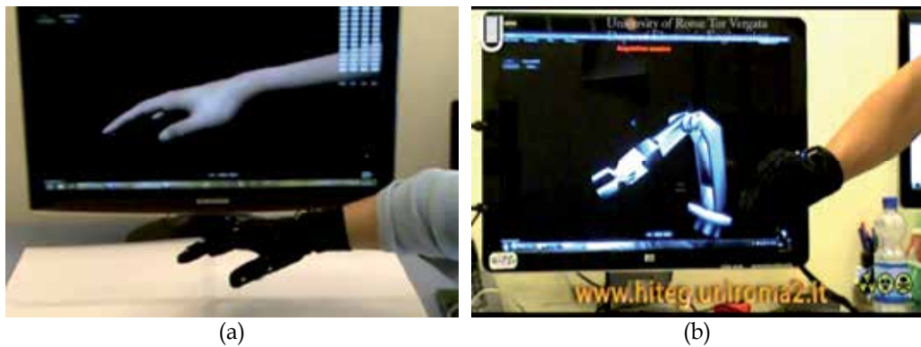
Fig. 15. Hiteg Data Glove measures human hand movements (a) simple reproduced on a computer screen or (b) utilized to handle a virtual robotic arm.
