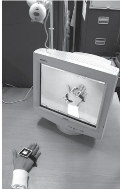
Fig. 6. AR arm rehabilitation using polished board, showing the virtual butterfly net superimposed on the image of the hand.
