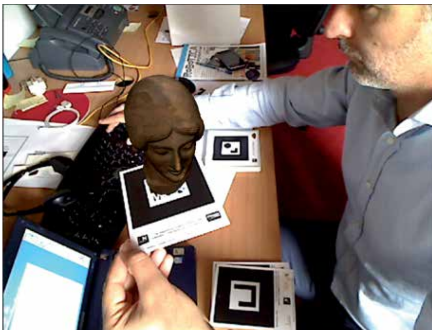
Fig. 4. An example of marker-based AR desktop session with a simplified 3D model of an ancient woman's head. The model was created using data derived from 3D laser scanner.
