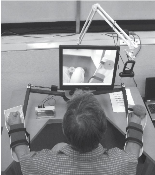
Fig. 4. Able-B to allow an individual to exercise their hemiparetic right arm, using AR to show their hemiparetic arm interacting with a computer game.
