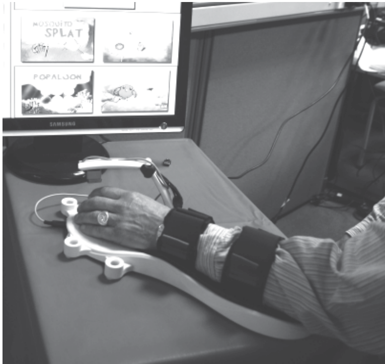
Fig. 7. Able-M, a gravity supported arm exercise device that interacts with computer games.
