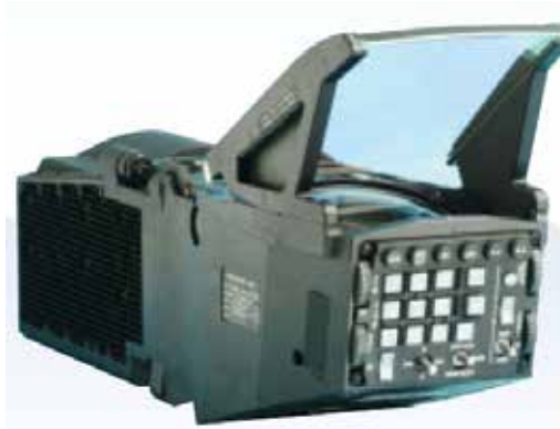
Fig. 23. A type of head-up display system.
